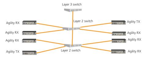
A significant requirement in line cascades is the need for sizable bandwidth between the switches in order to provide redundancy and in so doing prevent data bottlenecks. When linking 48 port switches, generally a 20 GB link bandwidth is required between the multicast router and the first switch. A 10 GB link bandwidth is then required between the first and second switches. The reason for this becomes clearer when data paths are added to the diagram.
