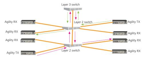
The streaming output from any transmitting device must travel up to the Querier, even if a recipient is located on the same switch as the transmitter. Given that the top layer 2 switch must also pass up and down all data from the lower switch, this is the reason for its double bandwidth link with the L3 switch.
