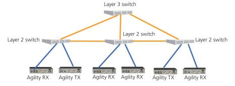
The advantage of arranging switches as a line cascade is that the communication links between them effectively form a simple bus structure that avoids the IGMP traps encountered by the pyramid arrangement.
