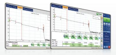
This improved version of linear view provides the flexibility to display both the OTDR graph and its linear view without having to toggle to analyze your fiber link.
