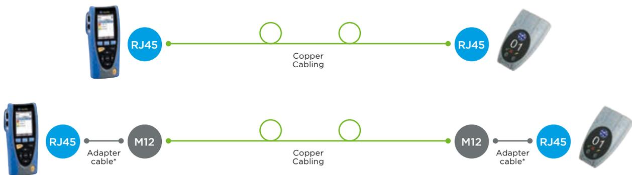
2 x M12 D connector cables supplied as standard.
