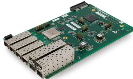
The new 1GE/100M/10GE expansion module provides 1GE fanout and 10GE support. The module features 4 SFP and 4 SFP+ ports to enable a combination of 4 100M and 4 1GE ports, or 8 1GE ports, or a combination of 4 1GE ports and 4 10GE ports. As networks evolve, 10GE has become more prevalent, so this internal fanout capability is critical to connect to newer network elements.
