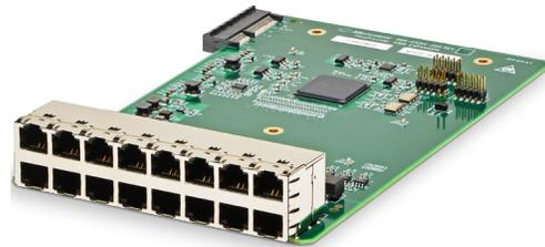
The E1/T1 internal module with 16 E1/T1 ports brings the unit to a total maximum of 20 E1/T1 ports (4 in base and 16 in expansion module).
