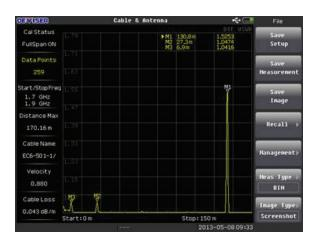
**Interference Analysis** can detect signal as low as -152 dBm and supports spectrogram display, RSSI, signal strength and signal ID capabilities.
