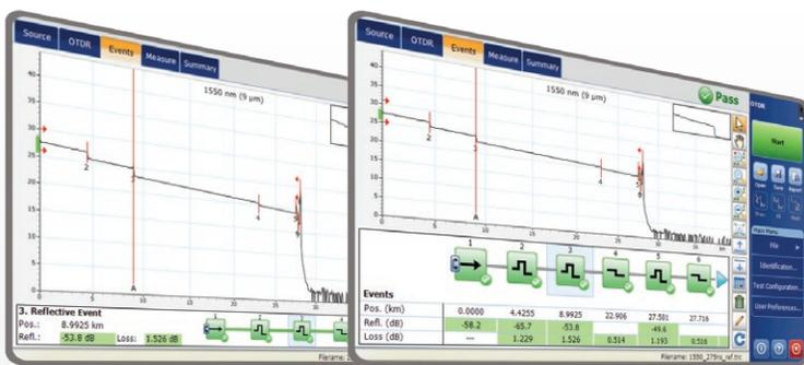
This improved version of linear view provides the flexibility to display both the OTDR graph and its linear view without having to toggle to analyze your fiber link.
