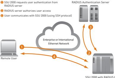
SSU 2000 with RADIUS Capable Communication Card
