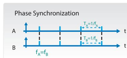
Leading edge of the pulses are at the identical moment.
