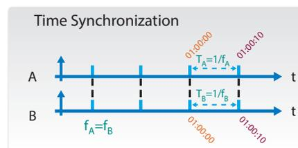
Leading edge of the pulses are at the identical moment and identical time.
