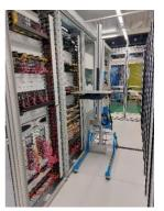
In addition to lifters for handling servers, we have also developed a range for batteries that can also be used for servers with smaller loads.
