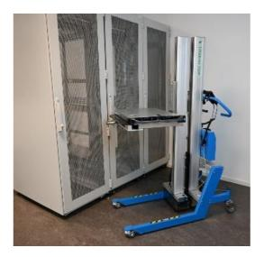
The Lift&Drive DC 15 U52 is equipped with a telescopic column with a sliding platform to facilitate the picking up and placing of a server. This lifting device has a minimum height from the floor of 95 mm and a maximum height of 2459 mm.
