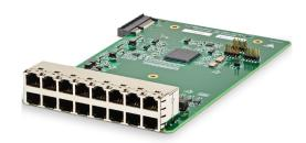
The E1/T1 internal module with 16 E1/T1 ports brings the unit to a total maximum of 20 E1/T1 ports (4 in base and 16 in expansion module).
