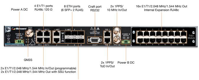
1x packet Ethernet In + management (with SyncE) - 1x RJ45 or 1x SFP cage. Either in-band management or out-of-band. 6x packet Ethernet Out (with SyncE) - 1x RJ45 and 5x SFP cage.
